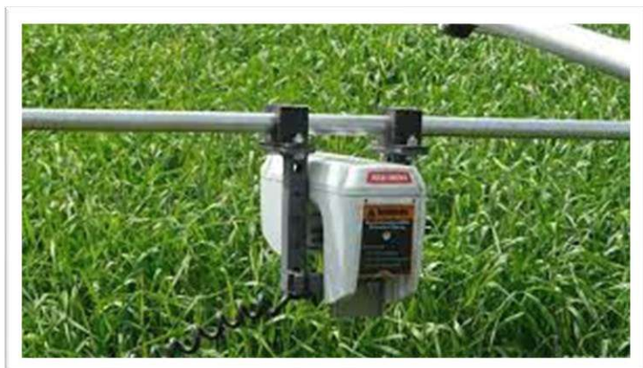
Fig. 17.7 Crop Sensor much fertilizer a plant may need, based on the amount of light reflected back to the sensor.
